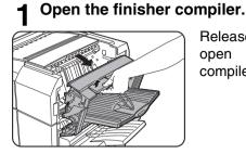
Release the latch to open the finisher compiler.
